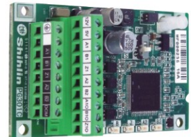
PG301C Speed feedback board (supports open collector type output)
